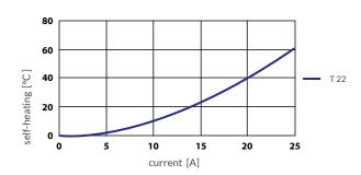
The characteristic curve in the diagram is measured with a thermal switch without any insulation in an oil bath.
